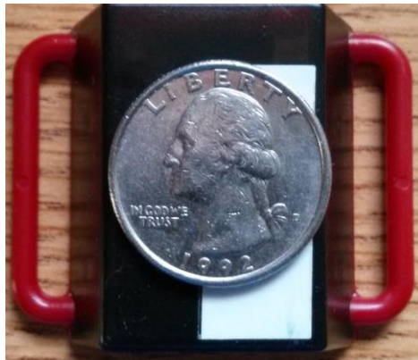
Figure 3-4 The Bluetooth IMU used for the experiments with a quarter for size reference
