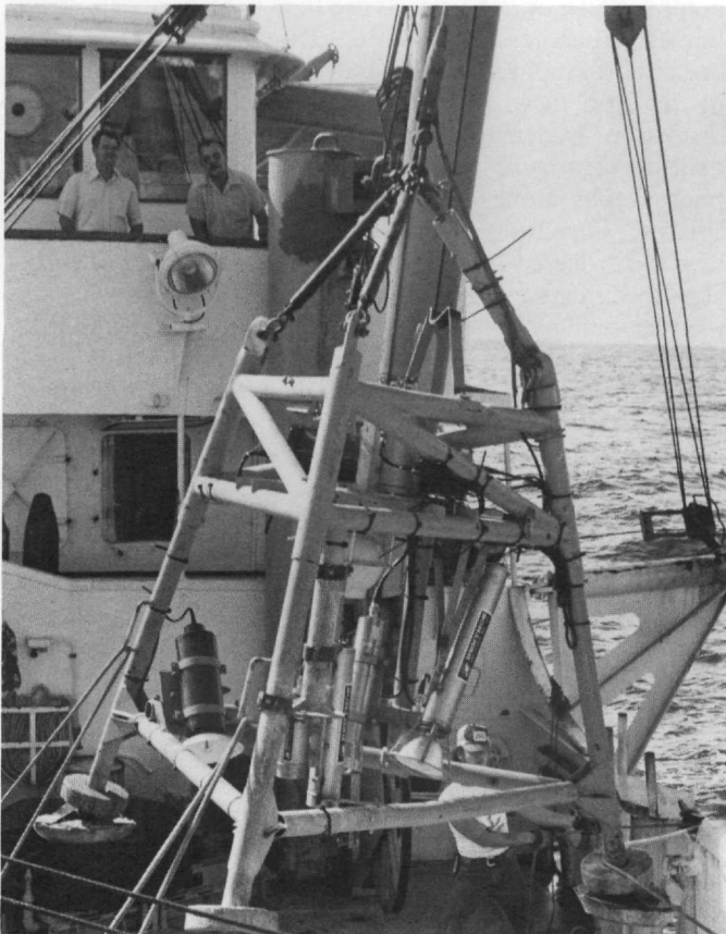
FIGURE 2. OMA/DVI deep submergence television survey system instrumentation mounted on tripod carrier vehicle.
