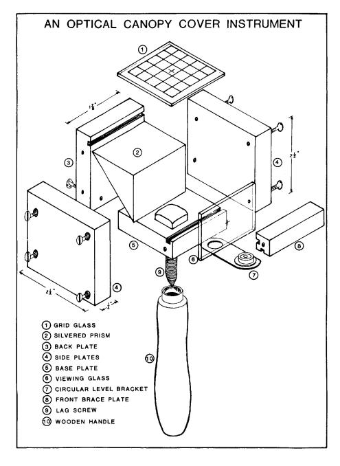
The right-angle silvered prism, the heart of the instrument, can readily be obtained from optical supply firms. Construction should begin only after the prism has been obtained to assure that the dimensions of the instrument are compatible with the size of the prism.
