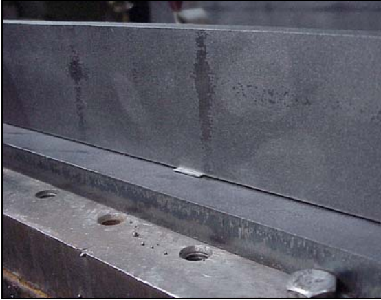
Figure 7 – T-joint displaying the insertion of shims in the experimental joint
