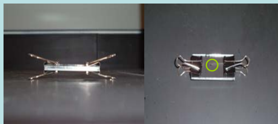
Figure 3: Profile view (left) of the analog apparatus and overhead view (right). Rhenium gasket is circled in the second photo. Dimensions of the slide are 46 mm x 26 mm x 2 mm and diameter of the gasket hole is 500 \mu m.
