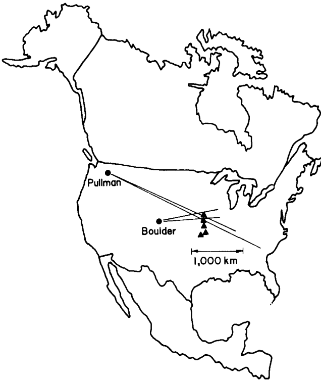
Fig. 11. Infrasound microphone arrays can track atmospheric disturbances several thousand miles from their sources. Two infrasound tracking stations ( circles ) follow the path of a severe thunderstorm ( triangles ). Two tracking stations are required, since the microphone arrays indicate direction, but not distance.
