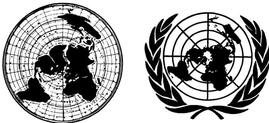
FIGURE 6. The original azimuthal equidistant projection known as Cassini's Planisphere. The map at the left centered on the north pole and extending to 60^\circ South Latitude was originally designed by Jean Domenique Cassini in 1679. The design at the right is the official symbol of the United Nations which uses as its central motif the azimuthal equidistant projection (Courtesy of Roy Wenzlick).
