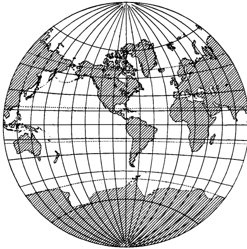
FIGURE 3. Van der Grinten's projection of the surface of the earth in a circular plane. The projection is neither equal-area nor conformal. (Drawn by Guy-Harold Smith).
