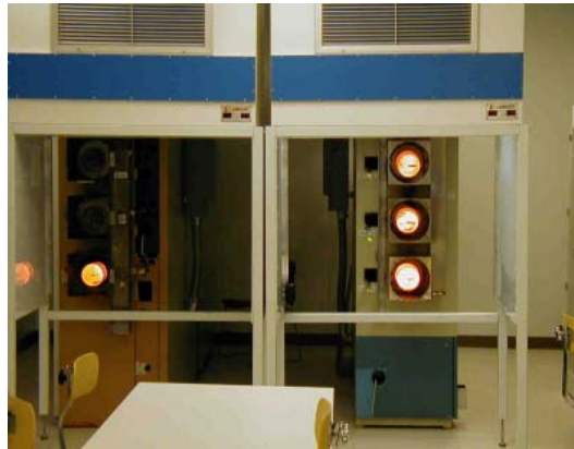
Figure 3.4: Furnace tubes for performing wafer oxidation and diffusion
