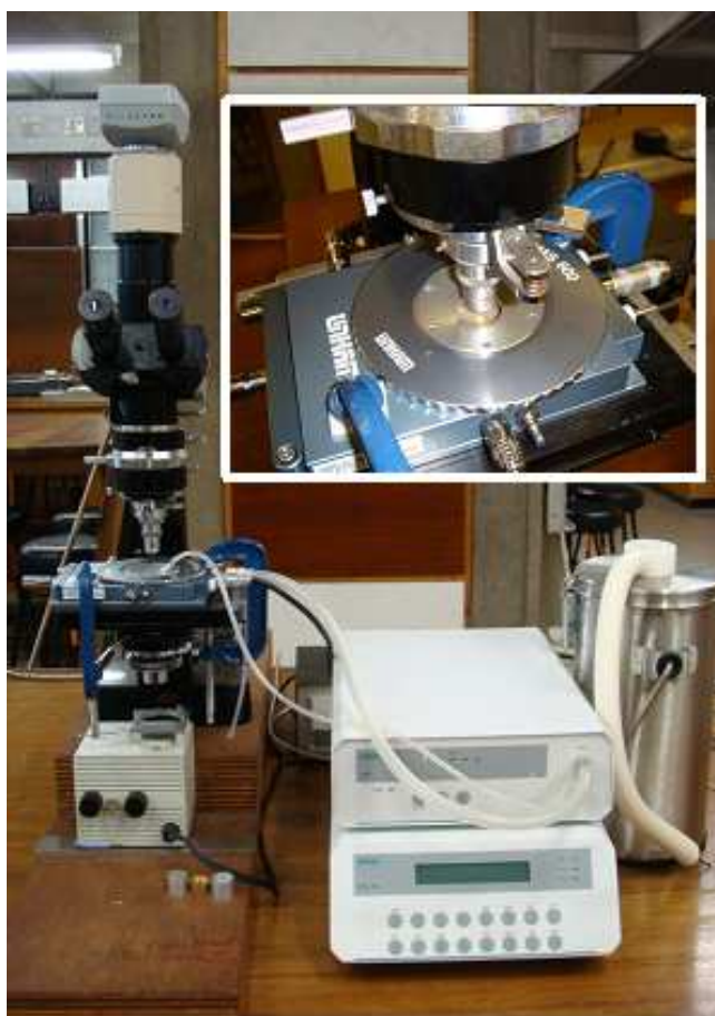
Figure 2.8: A Zeiss polarizing microscope equipped with a Linkam TMHS 600 hot stage (inset shows the hot-stage unit)
