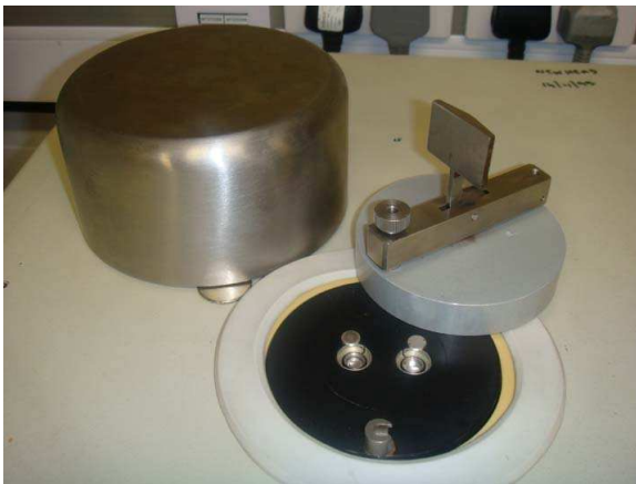
Figure 2.3: The photograph and schematic diagram of DSC head [74]
