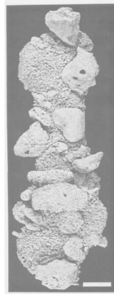
Figure 11. Mud layers recovered from near top of a buried interval of poorly sorted ooid sand facies in core D3 at a depth of 1.5m (4.9 ft)(scale bar = 2 cm).
