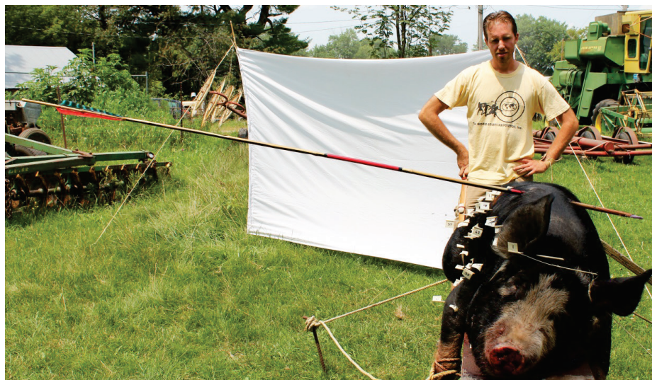
Figure 10. Dart shafts were marked with tri-colored fletches, stripes, and a 20 cm scale for video analysis. Shown here is shot # 64, which hit high and penetrated through the back.
