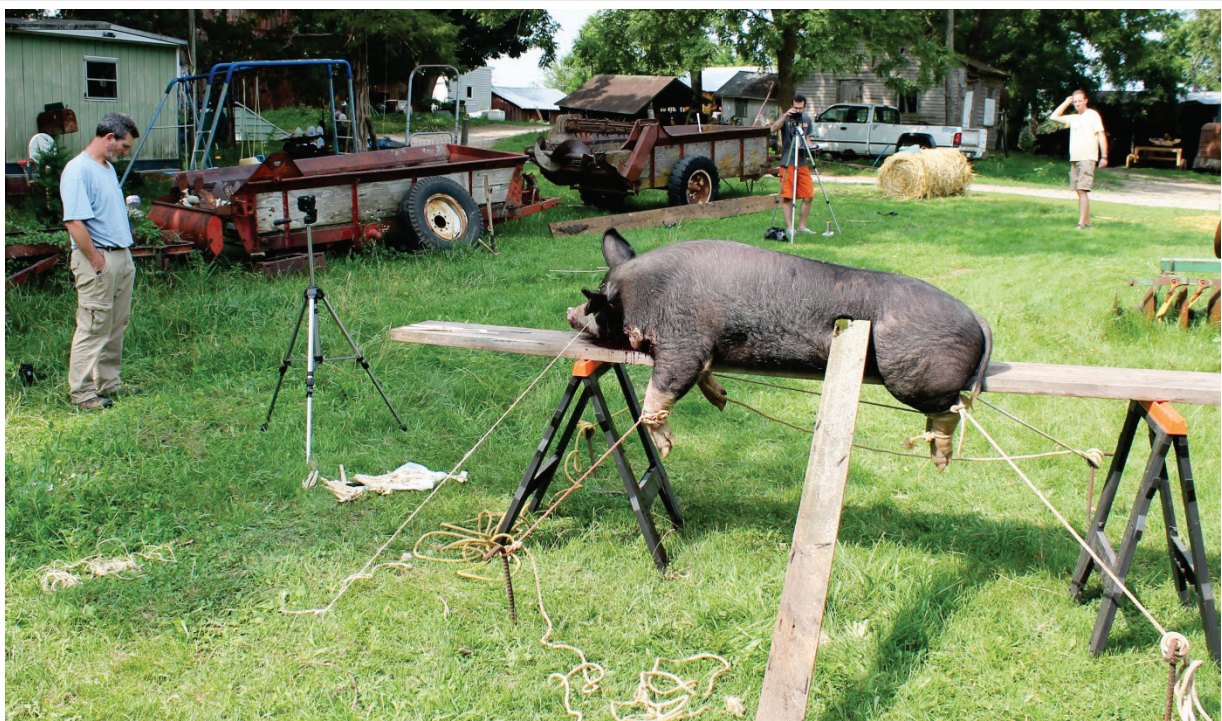
Figure 12. The setup of the experiment showing the method used to support the hog carcass.
