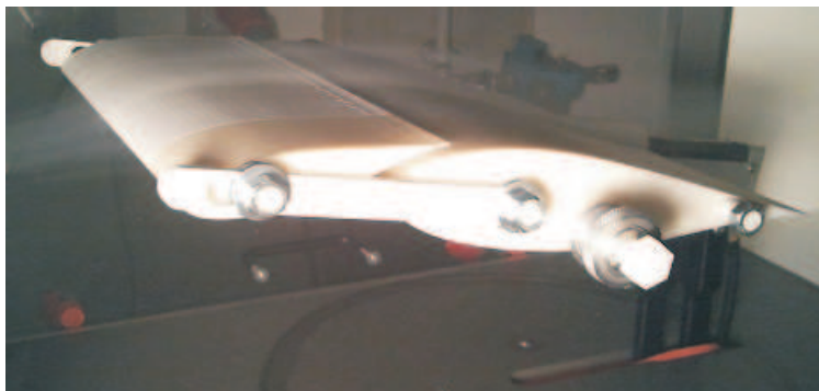
Figure 3.6 DU06-W200 double-element airfoil in the wind tunnel
