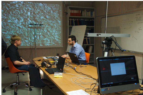
Fig. 2: The setup at the destination with the physical meeting room. The two locals were wearing hear-through devices including headpieces for the electromagnetic tracking system. The tracking system can be seen in the foreground of the image. In the back a big screen used to present the visitor can be seen.
