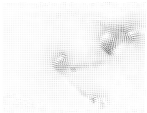
Figure 9: Vortex created 1402ms after plate release.
