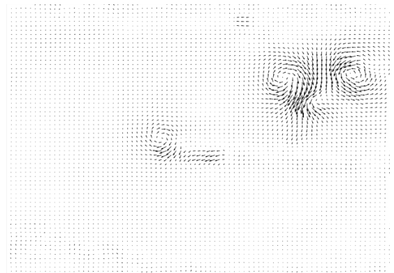
Figure 8: Vortex created 1088 ms after plate release.
