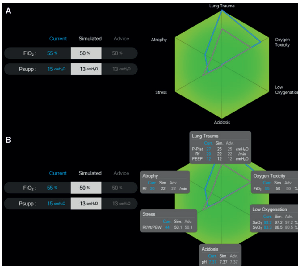
Figure 5: Simulation user interface of Beacon following a piece of advice for a single patient, without (5A) and with (5B) surrogate variables displayed.
