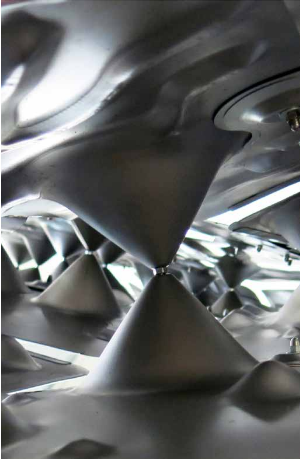
Figure 8: Interior view between upper and lower skins showing formed connections and patterning.
