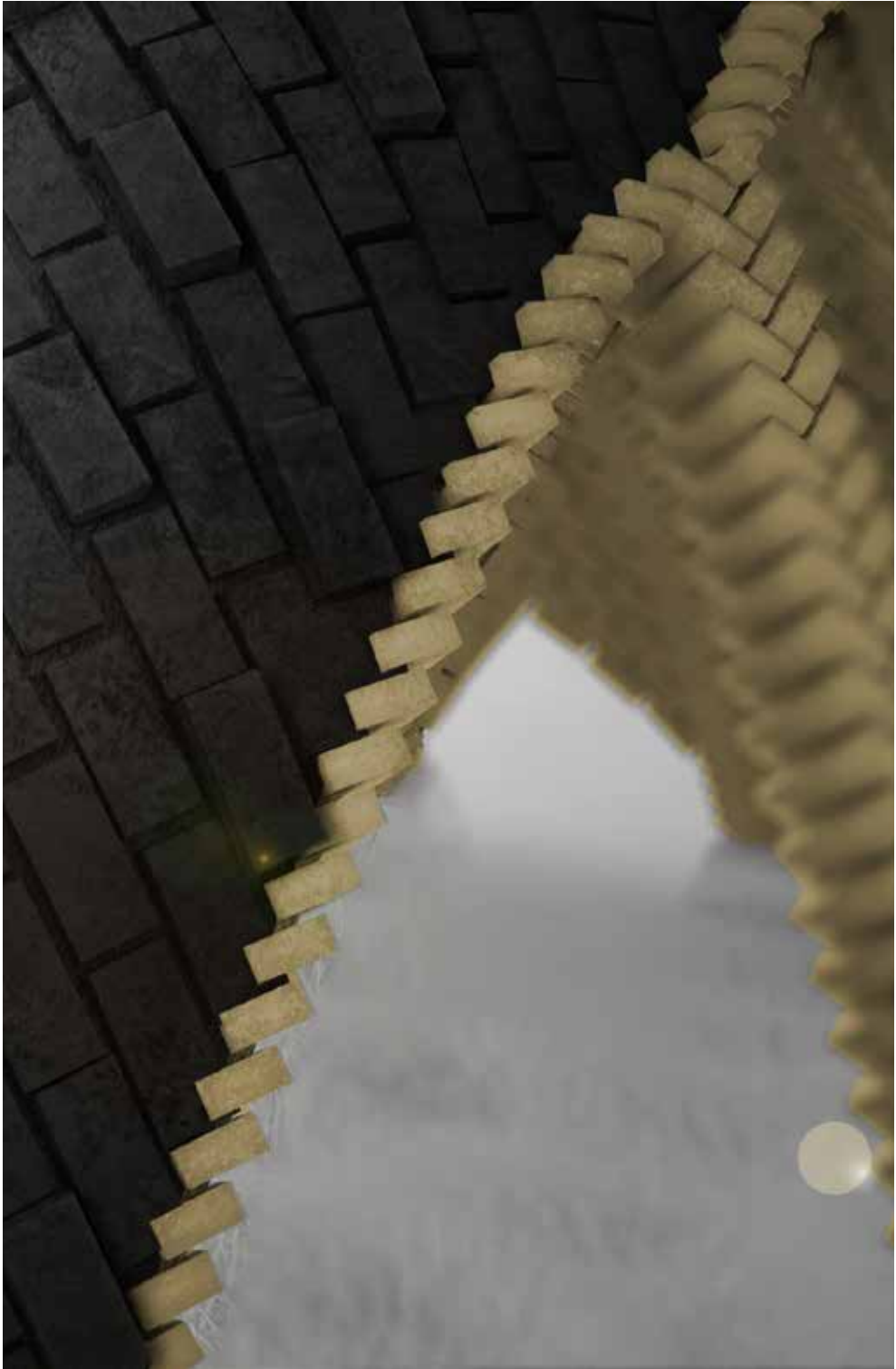
Figure 6: Rendering of pavillon assembly with outer layer of vaults in dark brick and inner vault layer and arches in light brick.
