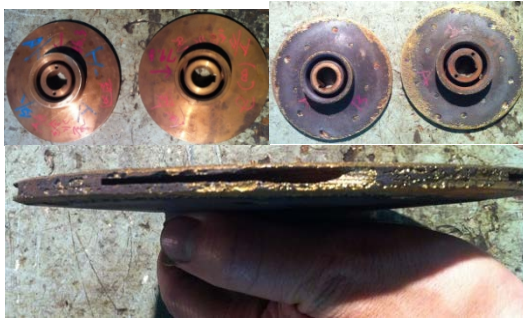
(upper left part shows new product, upper right part shows old product, lower part shows abrasion)
