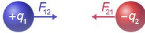
Fig1: Two charged particles are accelerated in each other electric field (without connection)
