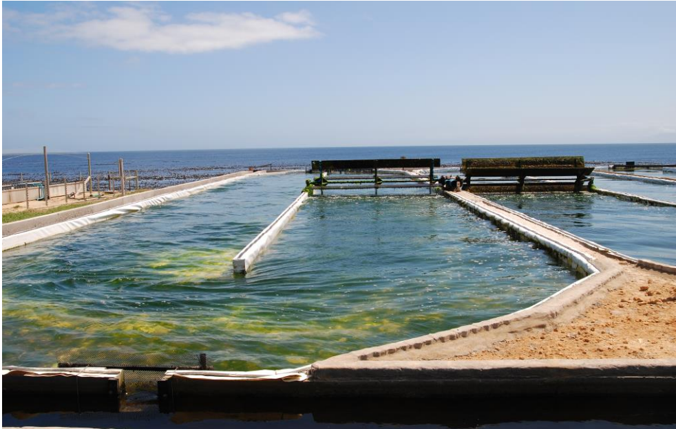
Figure 1: Flow-through, paddle-wheel raceways are the preferred method for growing Ulva .
