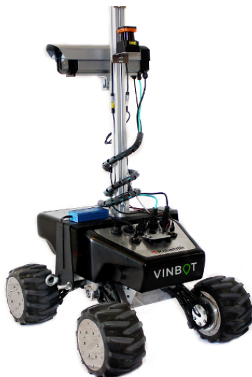
Figure 1. View of the actual version of the Vinbot robot platform
