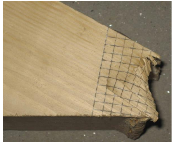
Figures 29 and 30 – Crushing at the front-notch surface concerning in the rafter and tie beam side without gap (left). Crushing at the front-notch surface of the rafter with an initial gap (right).
