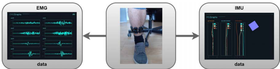
Fig. 2. Exploratory experiment with Myo device placed in a person's leg. Similarly to what occurs in an arm, Myo bracelet is also capable of acquiring EMG and IMU data from a leg. It was noticed that several leg gestures were suitable to be profiled due to the differentiation and consistency of acquired data.
