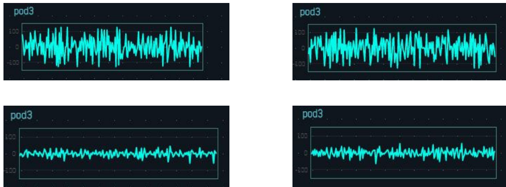
Fig. 4. Graphics showing the muscular activity of two repetitions of gestures A and B, obtained from Myo diagnostics page. The upper graphs are from gesture A, while the lower ones are from gesture B.
