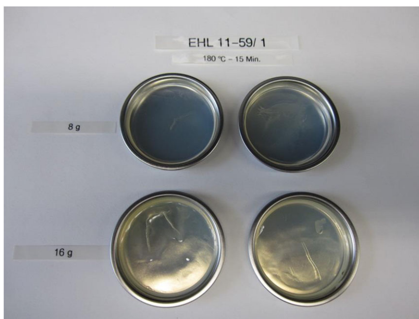
Figure 1. Photograph of 1,6-hexamethylenediisocyanate-based densely crosslinked polyisocyanurate samples.
