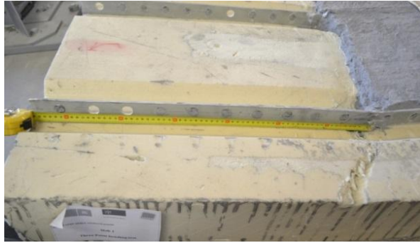
a) Damaged GFRP ribs after implementation of the experimental test in Slab 1
