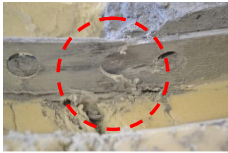
d) Experimental and numerical damage positions in the GFRP rib of Slab 1
