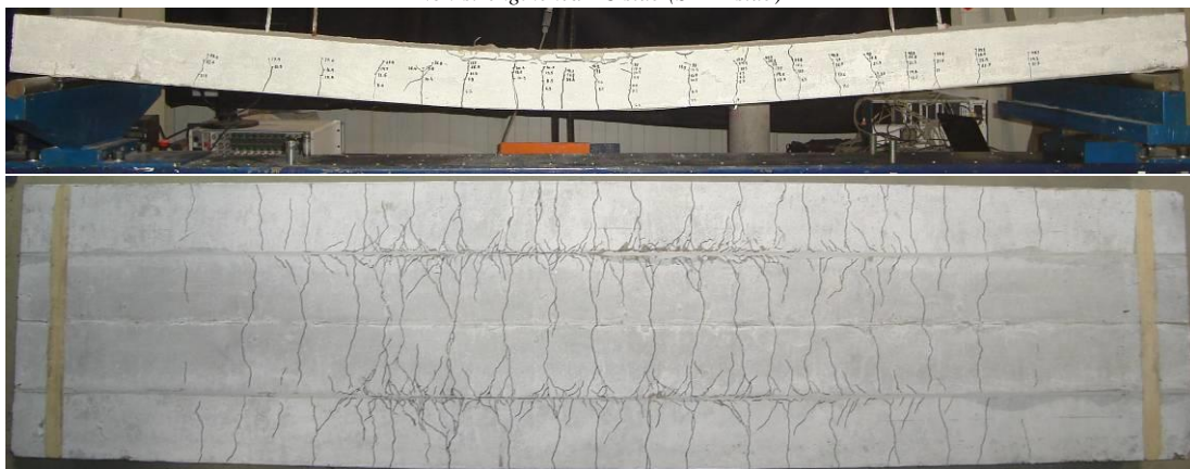
RC slab strengthened with non-prestressed CFRP laminates (S2L-0 slab)
