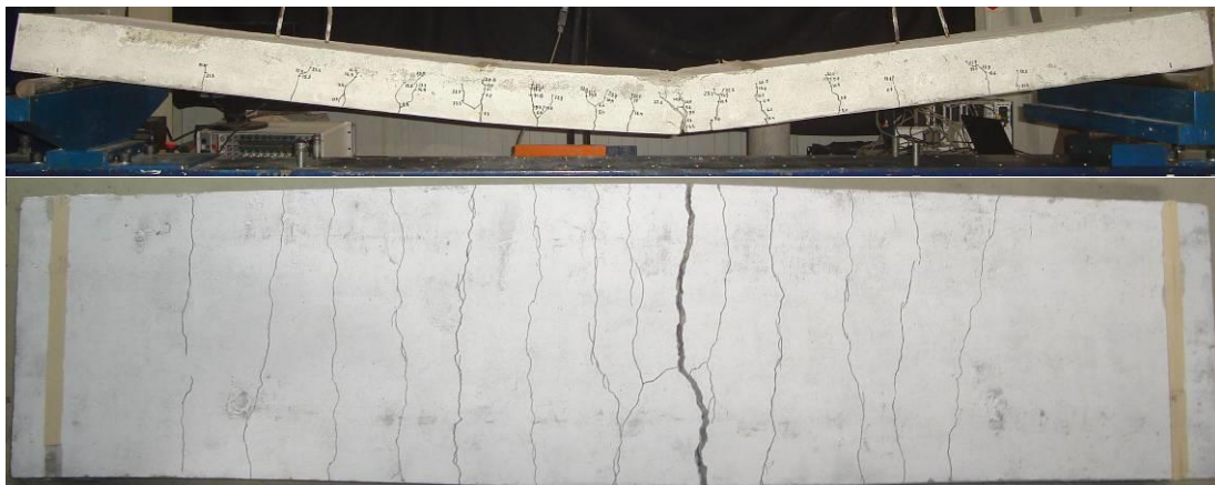
Non-strengthened RC slab (SREF slab)
