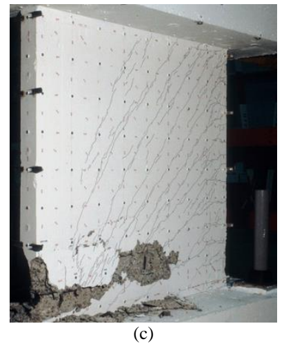
Fig. 16 – Simulation of the shear walls S1, S2, S4, S9, S10 tested by Maier and Thürlimann [29]: (a) horizontal load versus horizontal displacement relationship, F_h-U_h ; (b) numerical crack pattern predicted by PDSC model and corresponding to the final converged step; (c) experimentally observed crack pattern [29].
