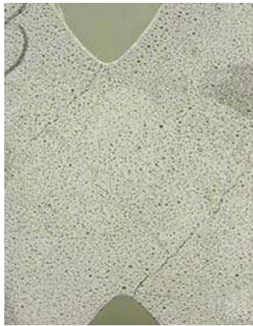
b) final crack pattern of PCM
