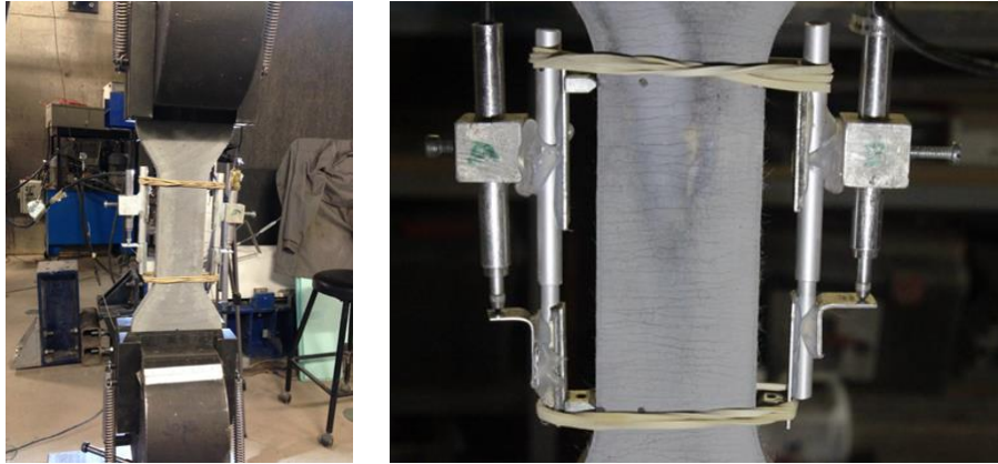
Fig. 2-Test setup used for the tensile tests.
