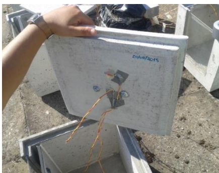
Fig. 1 – type K thermocouples placed on cover
