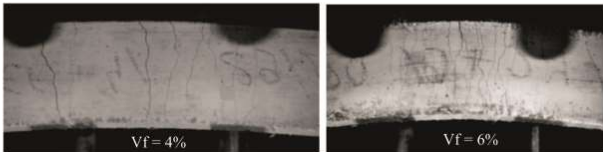
Figure 11. Effect of fiber volume on cracking pattern
