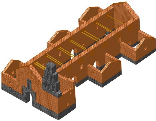
Figure 6. Finite element model of the church
