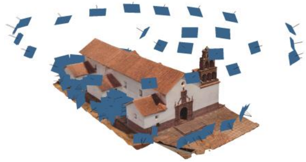
Figure 2. Image acquisition for photogrammetric 3D reconstruction of the church of ‘San Juan Bautista de Huaró’
