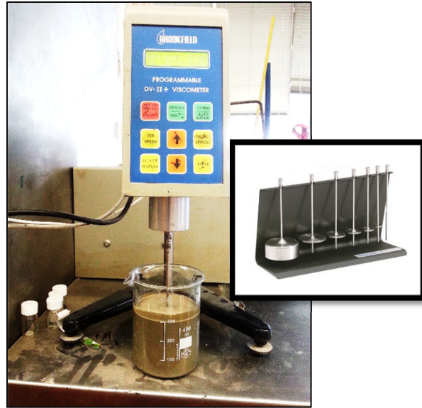
Figure 3.25: Typical Brookfield viscometer and its spindles.
