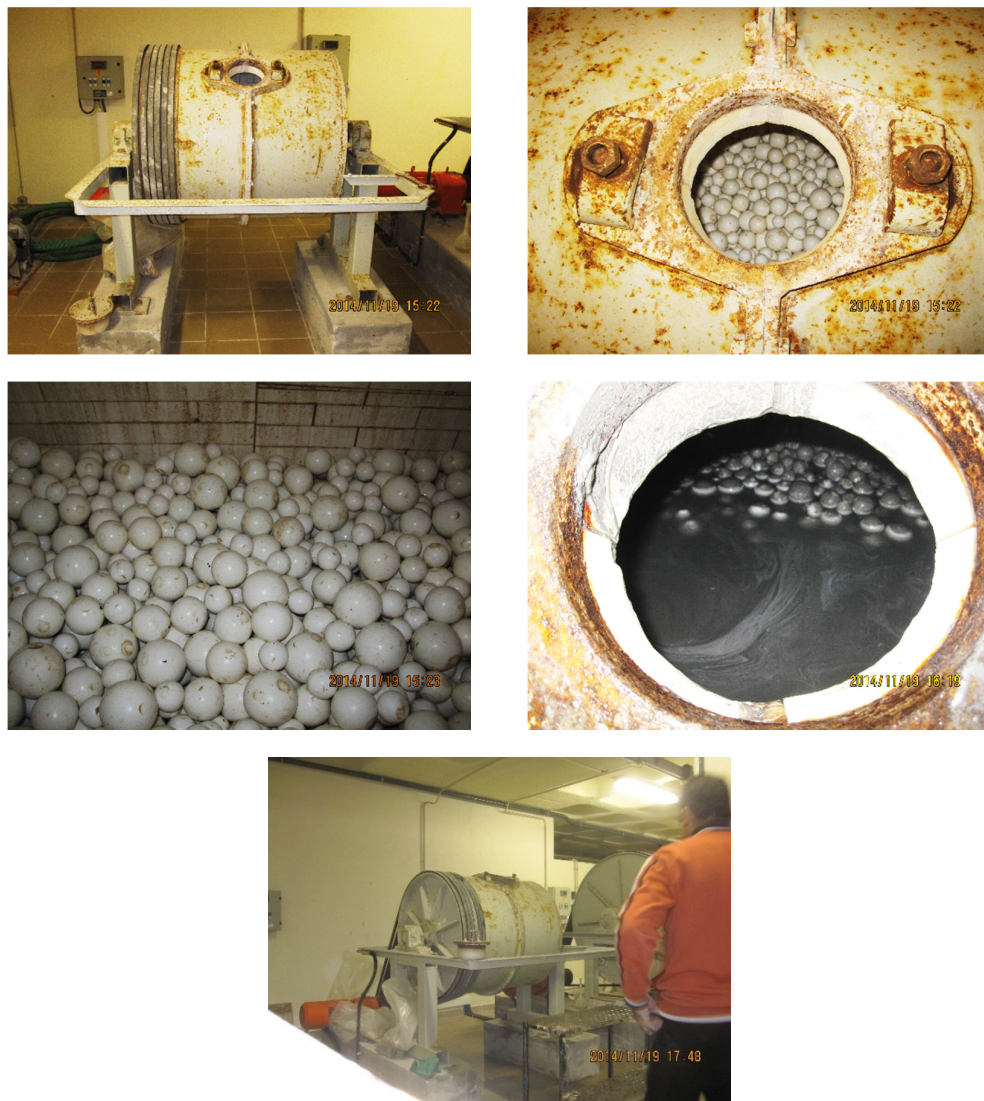
Figure 3.19: Wet-milling machine with 100 kg capacity
