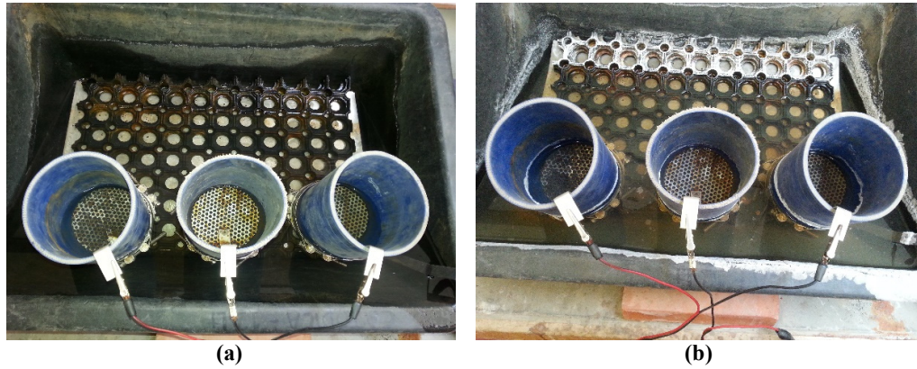
Figure 5.24: The cathodic solution at the beginning (a) and after 14 days in 60 V (b).
