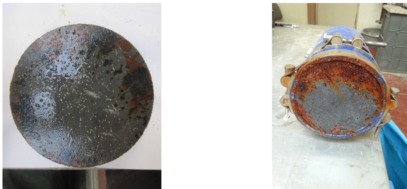
Figure 5.23: corrosion of specimens' surface.
