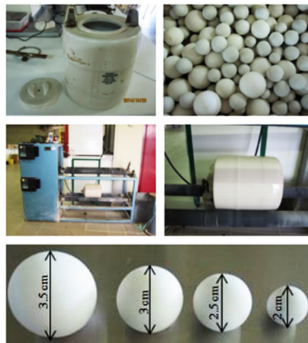
Figure 3.11: Wet-milling machine and its ceramic balls.
