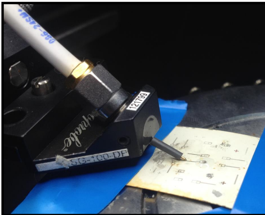
Figure 6.20 Three point probe connected to the VNA, touching the modified CPW.
