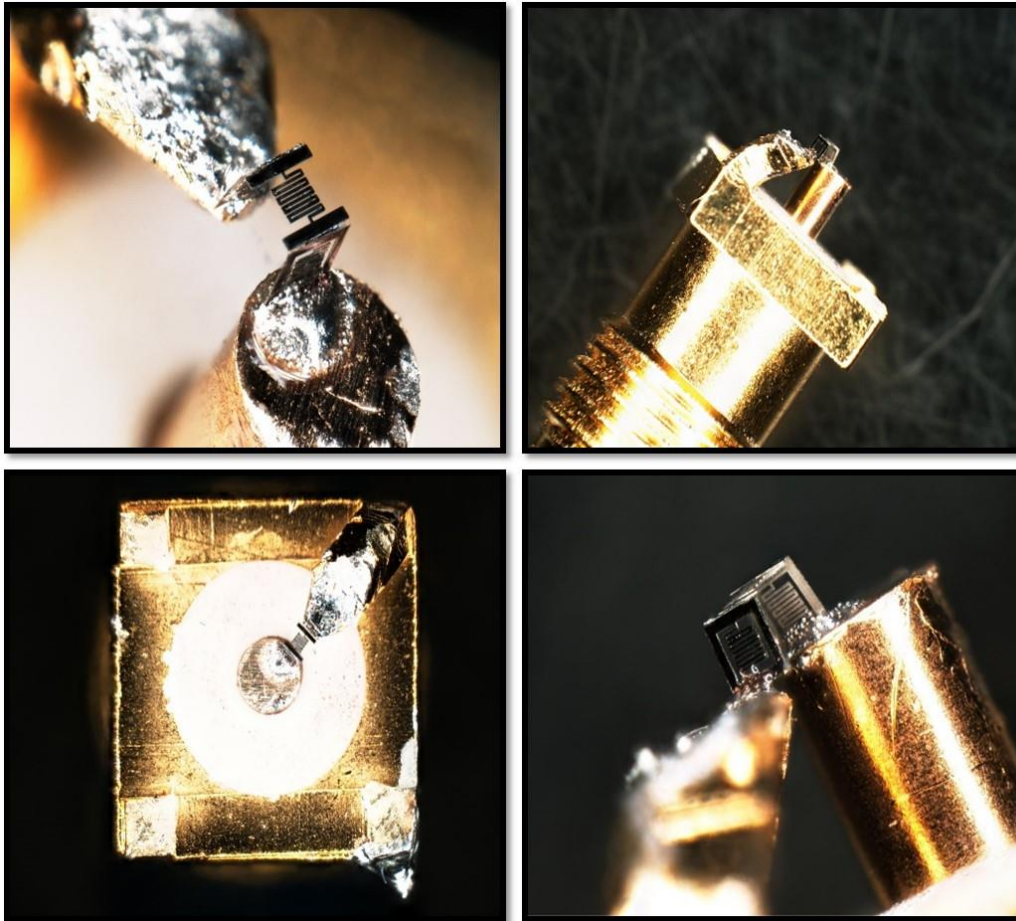
Figure 6.4 Micro antenna soldered to a modified SMA connector.
