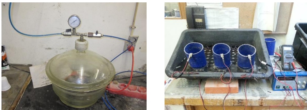
Figure 3: Chloride-ion- migration test setup.
