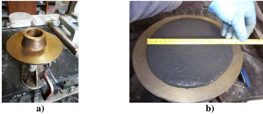
Figure 2: Flow table test apparatus (a) and flow diameter after test (b).
