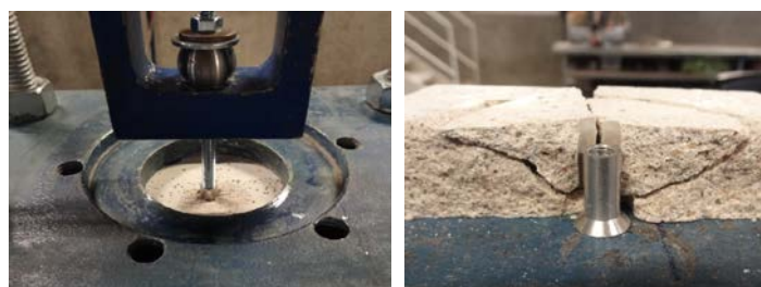
Figure 10: Test pullout body of internal thread (left) cylindrical configuration with slip (right) pullout test of conical insert
