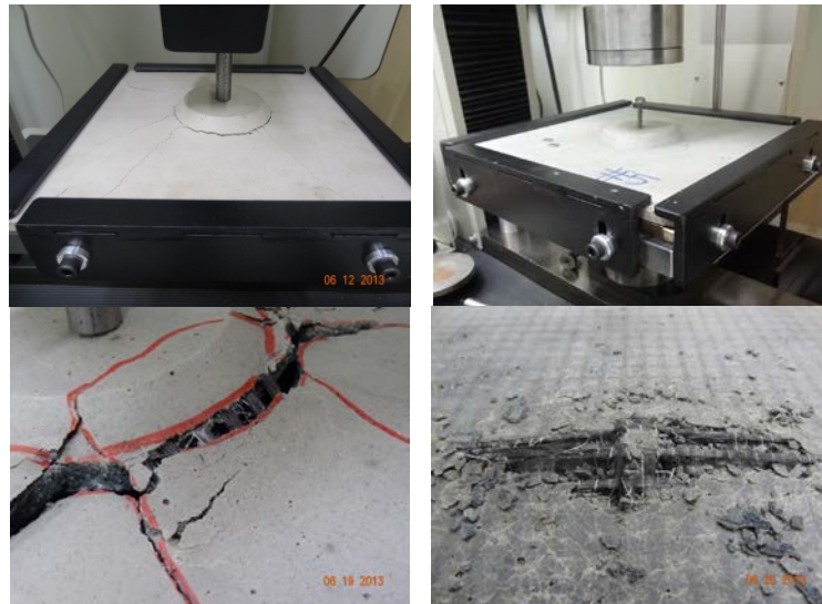
Figure 13: Bending test plate (left) traction punching and rupture mode (right) compression punching and rupture mode
