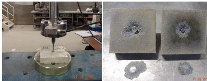
Figure 12: Pull-off test of metallic body (left) configuration the test (right) push-off inverted cone for the two configurations
