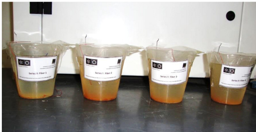
Fig. 4. Immersion of steel fiber in 3.5% NaCl solution during 7 days.
