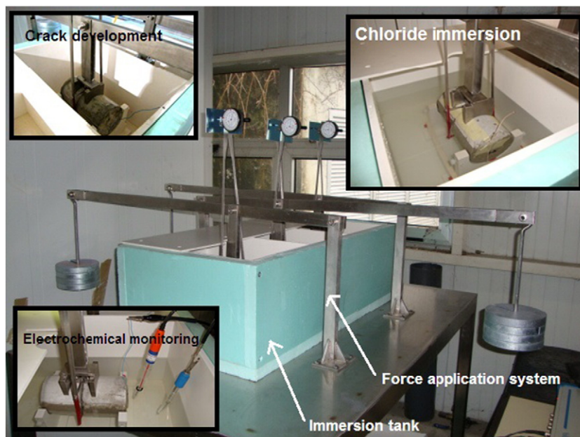
Fig. 6. Chloride immersion of cracked specimens under tension.
