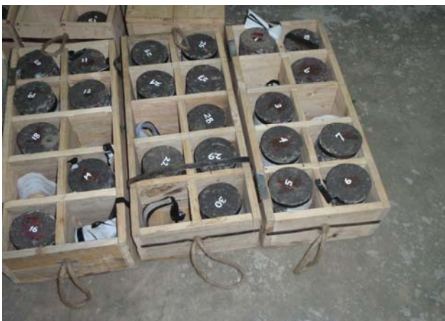
Plate 7.14(b): Some coring samples of bituminous layer that will be sent to testing laboratory
