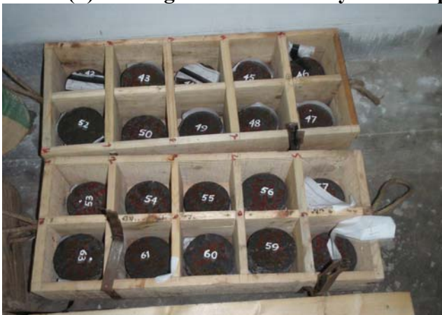
Plate 7.14 (a): Some coring samples of bituminous layer that will be sent to testing laboratory.
