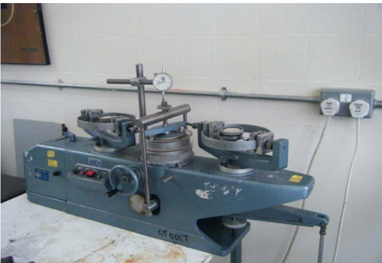
Plate 7.7: A picture of ring shear apparatus for determination of residual shear strength of remoulded soil
