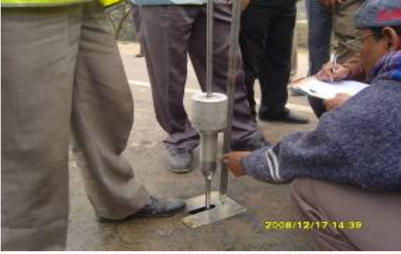
Plate 7.15: DCP test at core location N4 road.
