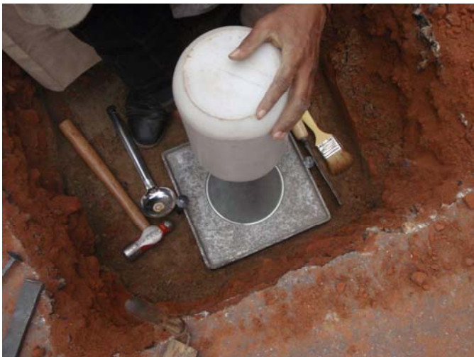
Plate 7.18: In situ density by sand replacement method of base layer of pavement at R301
