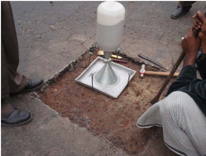
Plate 7.18: In situ density by sand replacement method of base layer of pavement at R301
