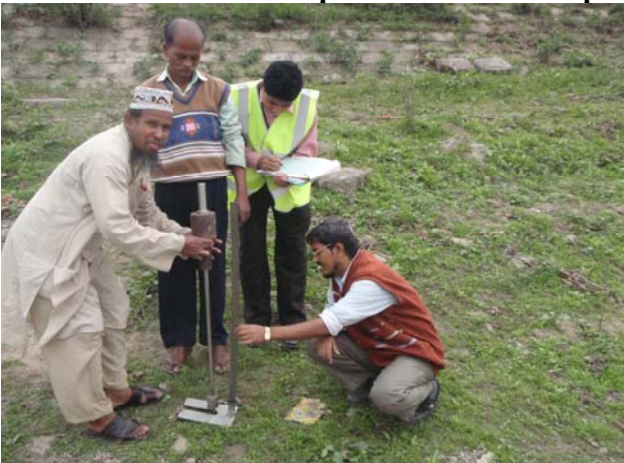
Plate 7.17 (a): DCP test done at toe of Embankment of Tongi – Ashulia – EPZ Road
