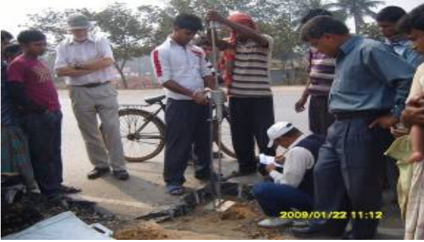
Plate 7.16: DCP test at pit location from top of granular base layer of N4 road.
