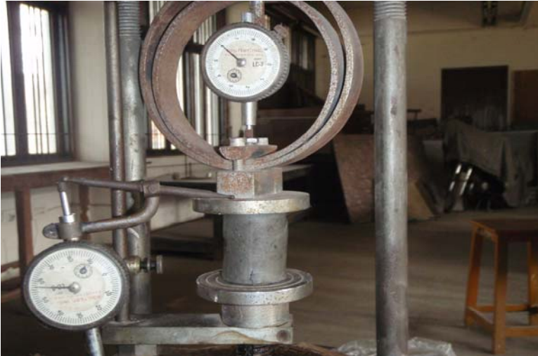
Plate 7.2: The Unconfined Compressive Strength equipment and tested soil samples during operation of the test
