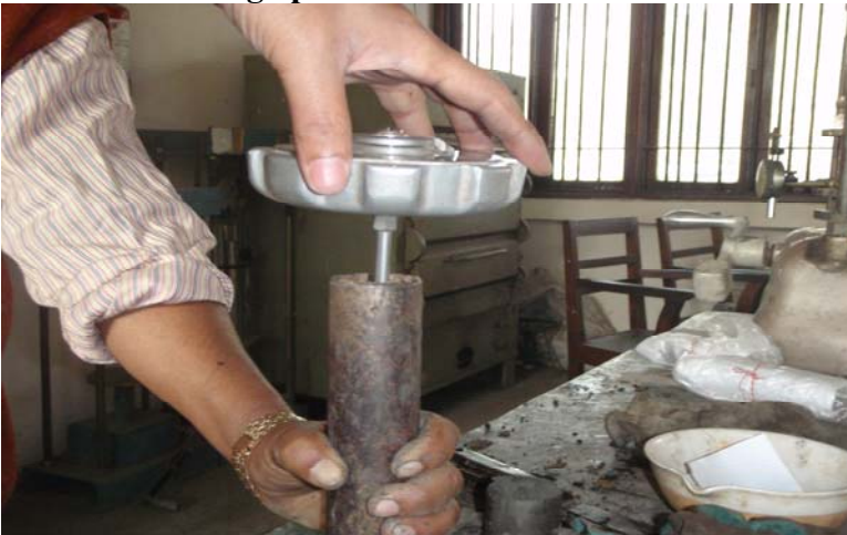
Plate 7.3: Laboratory Hand Vane shear test for undisturbed soil samples collected from different depths.
