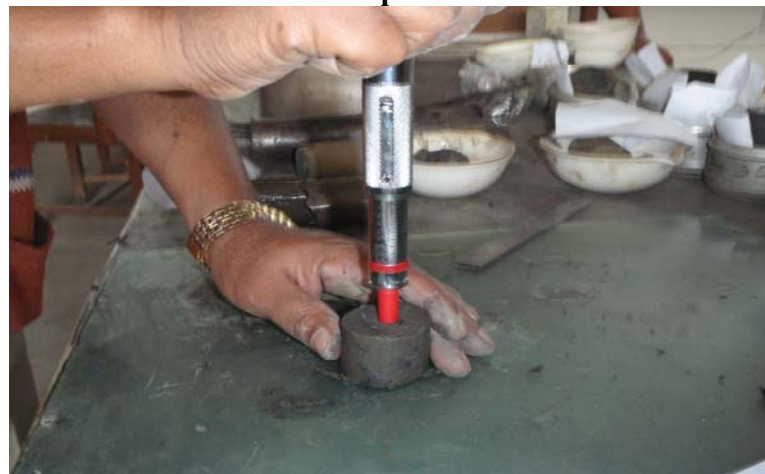
Plate 7.4: Use of Hand Penetrometer for measuring the undrained strength
