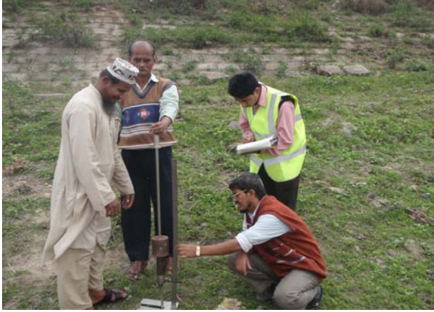
Plate 7.17 (b): DCP test done at toe of Embankment of Tongi – Ashulia – EPZ Road
