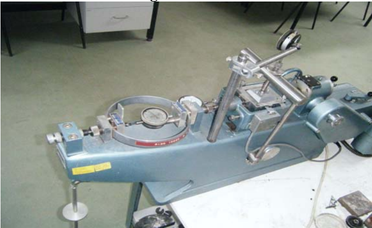
Plate 7.6: A Picture of Shear box apparatus used in performing direct shear box test
