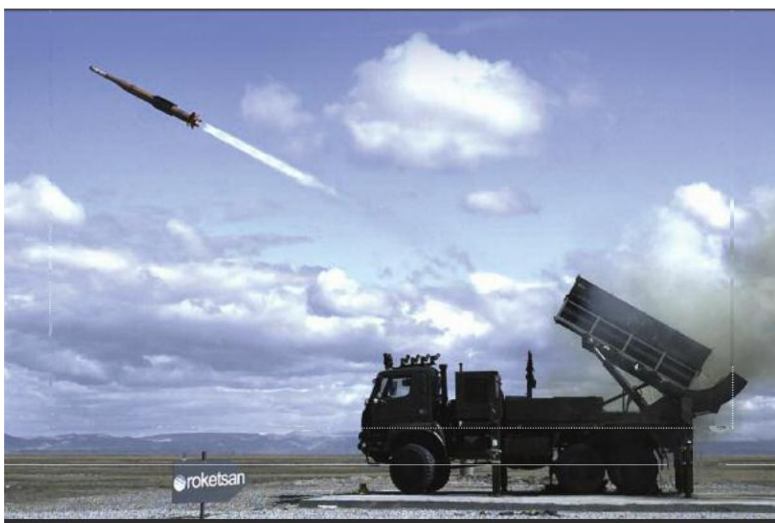
Figure 1.1 : Perchlorate is used in the missile systems in the Turkish Army. The combustible materials such as boron, magnesium and zirconium are mixed with oxidants such as potassium nitrate, PTFE or potassium perchlorate by using some polymeric binders (HİSAR-A, Low range anti-aircraft missile system, developed by ASELSAN and ROKETSAN)(Dinçer, 2014).
