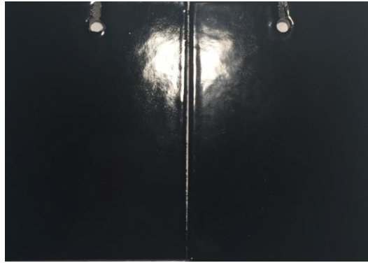
Figure 4.2 Coating on plastic component using pre- heating method
