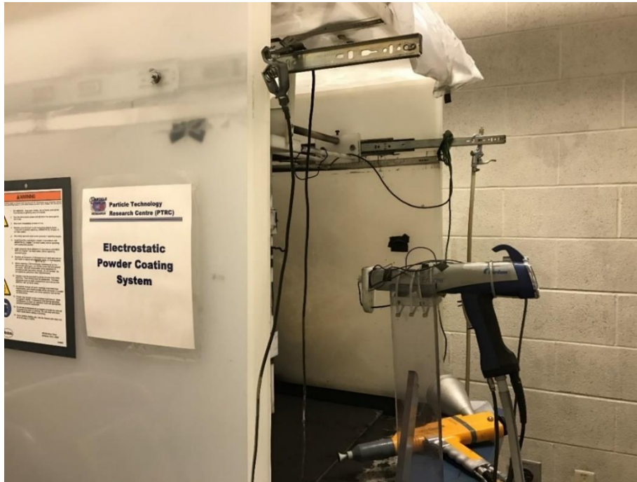
Figure 4.5 Nordson 902 Powder Coating Booth
