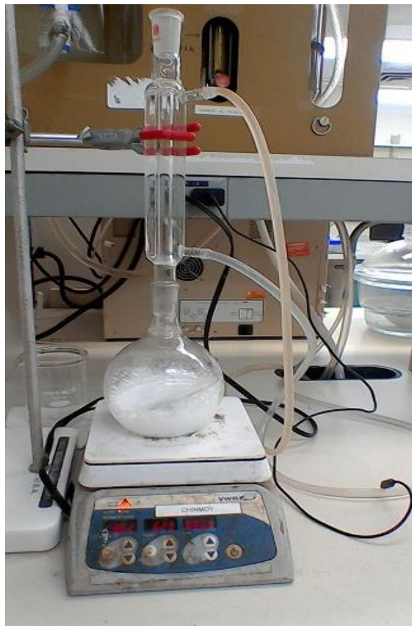
Figure 3.6: Preparation of PDMS Coating Solution using RTV 615: the mixture was continuously stirred and heated at 60°C to get a homogeneous cross-linked solution
