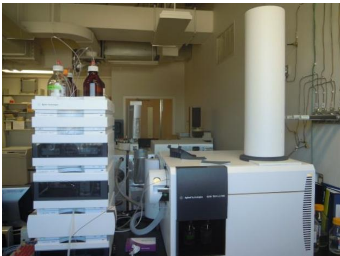
Figure 3.3: Agilent 6230 TOF-LC/MS used for EE2 Analysis
