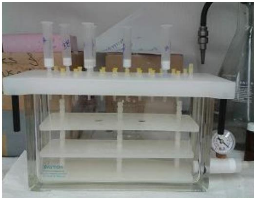
Figure 3.1: Solid-Phase Extraction of Water Sample using Hypersep C-18 Column
