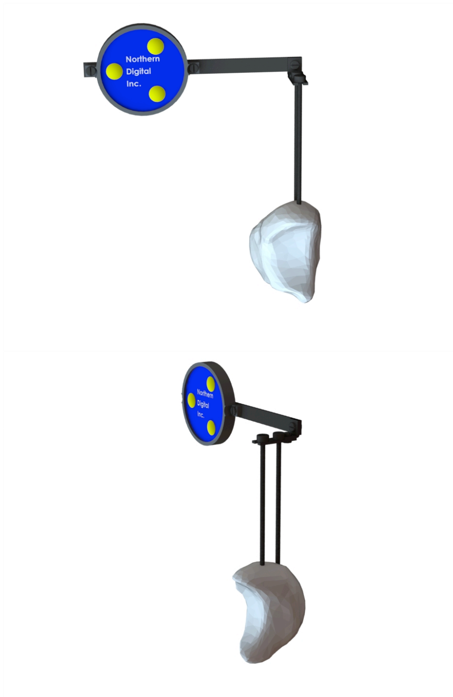
Figure B-2: Lunate Tracker Mount. Illustration of the lunate tracker mount inserted through a dorsal incision over the midpoint of the body. Secured with \varnothing 2.7mm cortical bone screws.
