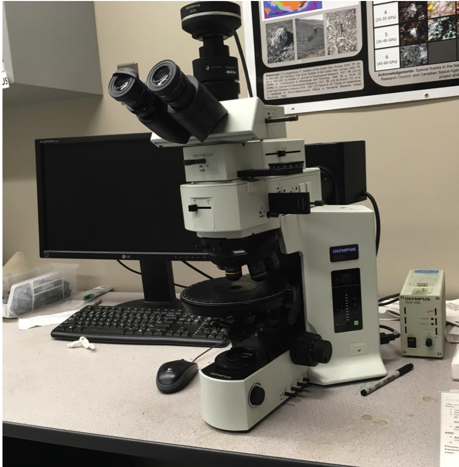
Figure 2.1. The Olympus BX51 microscope with attached Olympus UC30 high resolution digital camera used for petrographic observation
