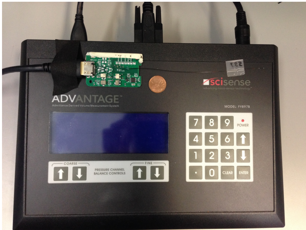
Figure 1.4: Commercial Pressure–Volume Tethered Measurement System from Transonic Scisense Inc. Interface Module, 1.2F Catheter, External Processing Unit [3].
