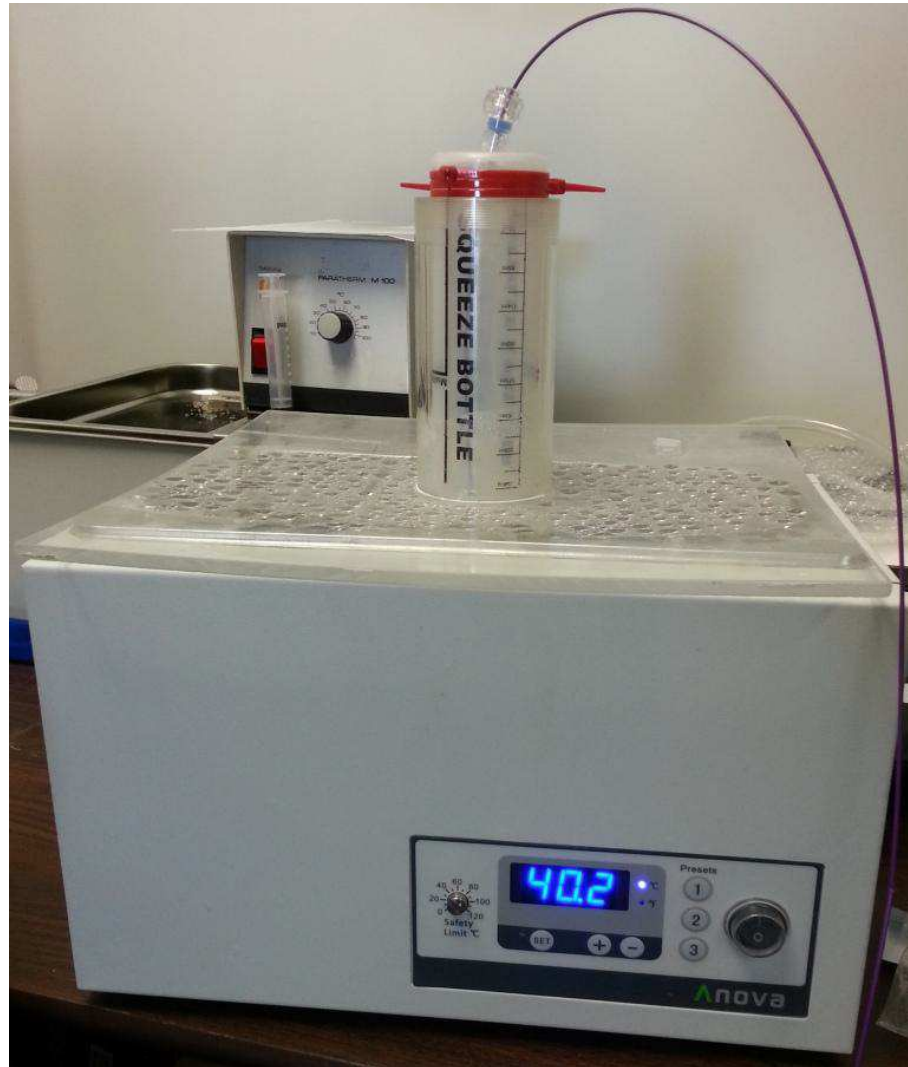
Figure 5.15: Experimental test setup – six liter water bath set to (40 \pm 0.2)^\circ\text{C} , implants are submersed into water and held there for the duration of the study.
