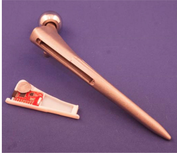
Figure 2.8: Smart hip implant proposed by [13]. Images from [13]. Copyright ©2016 IEEE.
