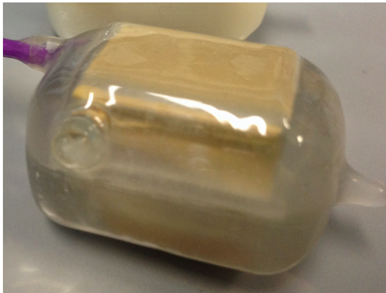
Figure 5.17: A closeup of the thick walled capsule 3D printed in RDG720 transparent acrylic material displaying internal chlorophenol water strips.
