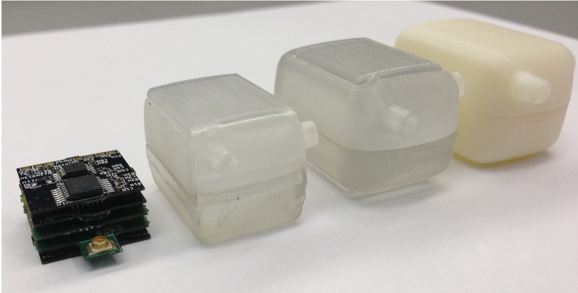
Figure 5.11: 3D Printed Plastic Packages for Pressure-Volume Implant from left to right: PV Telemetry system [30, 31], thin wall acrylic, thick wall acrylic, thick wall ABS-M30i (ABS not shown).
