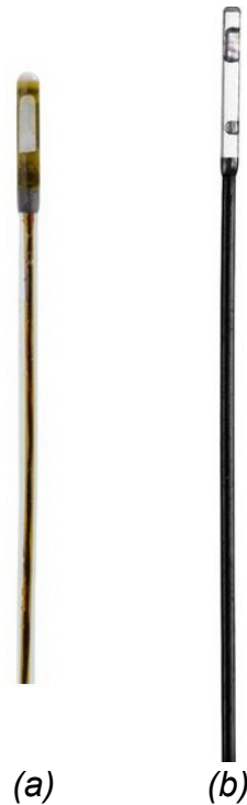
Figure 2.10: MEMS based pressure catheters for small animals from two manufacturers: a) Millar Inc. and b) Transonic Scisense.
