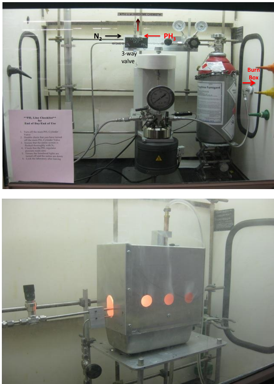
Figure A2.41. Photographs of the reaction setup (top) and burn box (bottom) used for the safe handling and disposal of PH 3 gas during this study.
