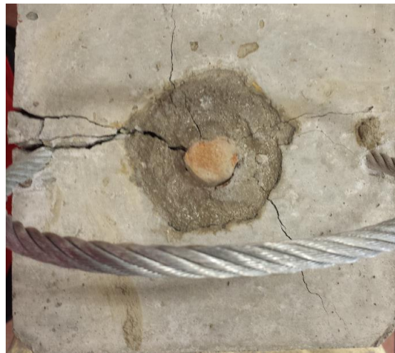
Figure 3.6: Tensile splitting through grout cylinder of specimen 12CN-1.
