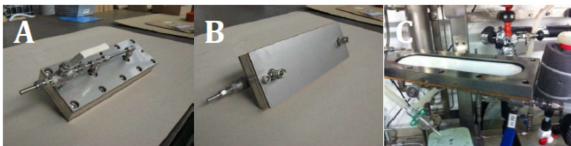
Figure D.1 Pervap 4060 membrane and test cell: (A) Assembled test cell showing permeate (vacuum) connection, (B) assembled test cell showing feed and retentate
