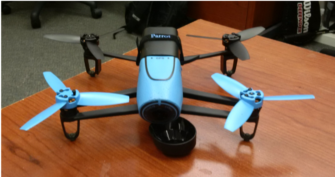
Figure 2.3: A commercially available drone, fitted with a fixed orientation 14 Mpixel fish-eye camera.
