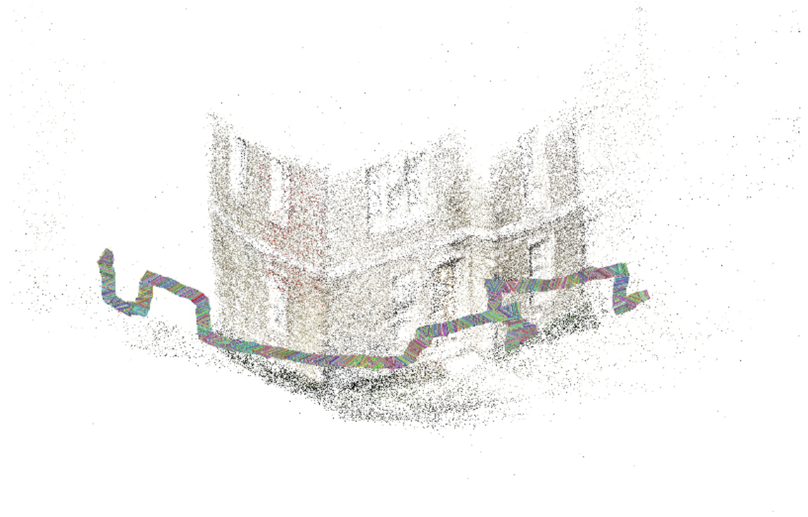
Figure 2.1: An example of a sparse point cloud, with the individual view positions and orientations visible (the snake-like structure).
