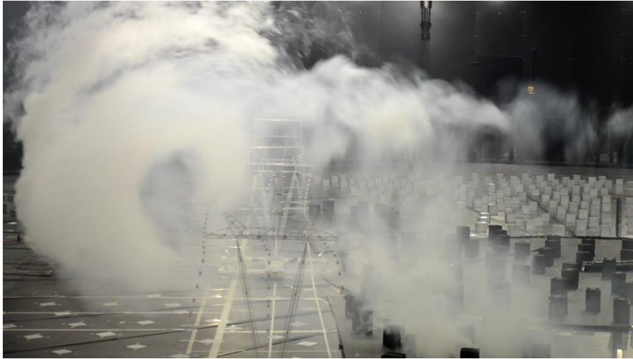
Fig. 3-4. Downburst formation snapshot at WindEEE
