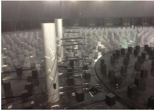
Fig. 3-5. Wind Field measurement using cobra probe devices
