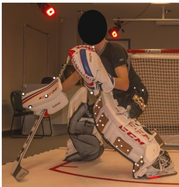
Figure 3.1: Markers located on the left pad, gloves, pelvis, thigh and leg. The leg rigid body was elevated 5 cm off the back of the shank so that it did not interfere with the goal pad straps.
