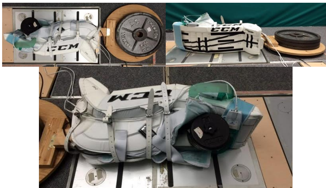
Figure 4.2: Setup for pressure sensor verification. The testing mechanism with load cell and effective mass were placed within the leg channel of the goal pad and fastened using the goal pad leg straps.
