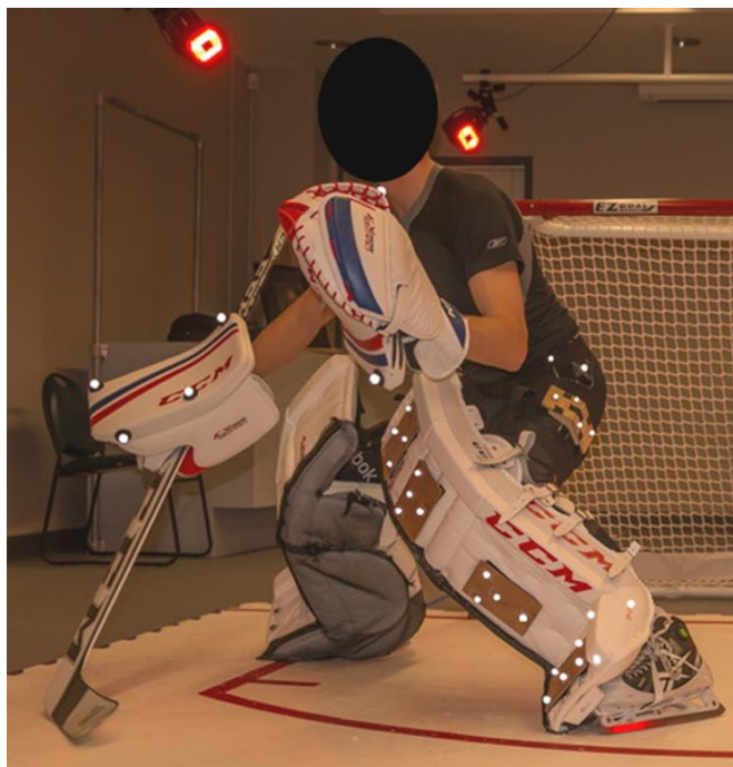
Figure 4.4: Kinematic marker setup on the goal pad (Thigh, knee, shin and boot with 3 individual markers located on the distal lateral aspect of each the left and right leg pad. Passive motion capture cameras are visible at the top of the figure and the synthetic ice with the goal crease inlay, used to replicate on-ice conditions, is visible at the bottom of the figure. The kinematic markers located on the gloves were visual and only used for tracking orientation.
