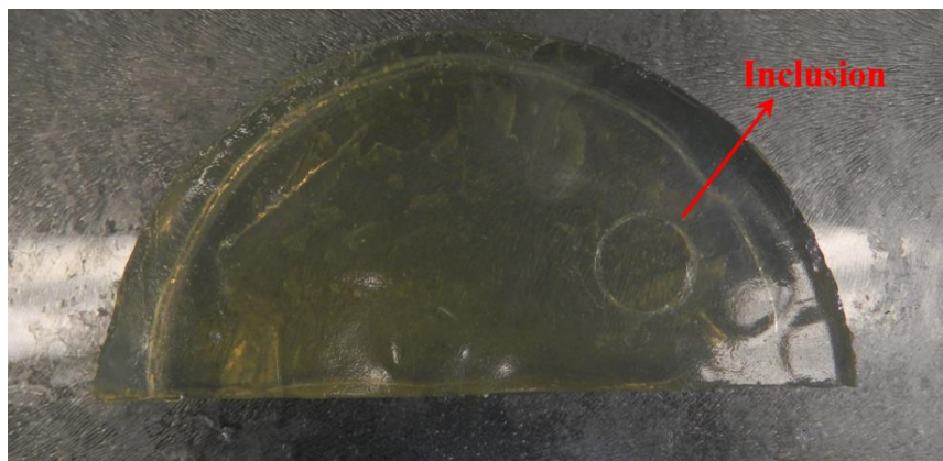
Figure 4.5. Gelatin breast phantom with inclusion located in the bottom right side to mimic the breast upper right quadrant.
